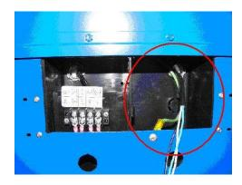
2. The connections are standard black, white, and green (ground). Replace the cover when complete.
