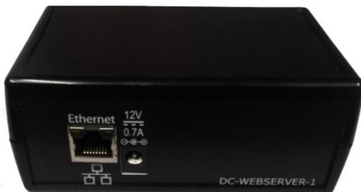
On the back of the DC-Webserver-Clocks-1 you will find connections for the Ethernet and the power.
