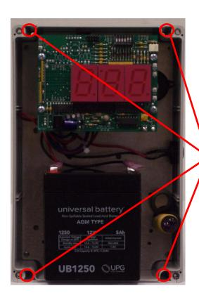
Remove the enclosure lid to gain access to these (4) .250 inch holes. This allows the unit to be mounted to a surface and still be protected by the gasketed enclosure lid.
