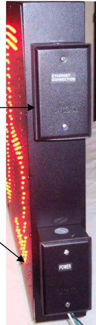
**Connections:** The DC-150N requires a breakered 120VAC @ 2 Amp, grounded and isolated electrical service.
